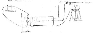
Conditions. — Large lead cylinder metallically connected with sheath of electrometer. Röntgen lamp surrounded by a lead sheath, which latter was also connected to electrometer sheath. There was a window in this lamp sheath 2.5 cm. broad and 5 cm. high. This window could be screened by aluminium or by lead. These screens were always connected metallically to sheaths. During all the experiments a Bunsen lamp was kept constantly burning, with its flame about 30 cm. below the Röntgen lamp.
