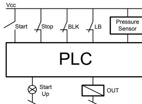
Figure 1. An example of a circuit signal connection
