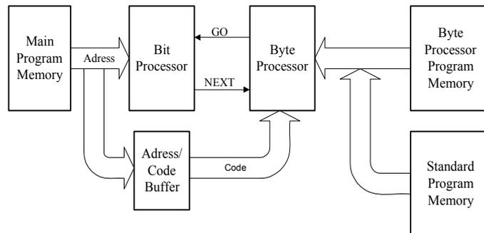
Figure 7. Bit-byte CPU with a master bit processor
