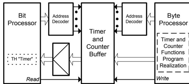
Figure 14. Realisation of the Timer and the Counter
