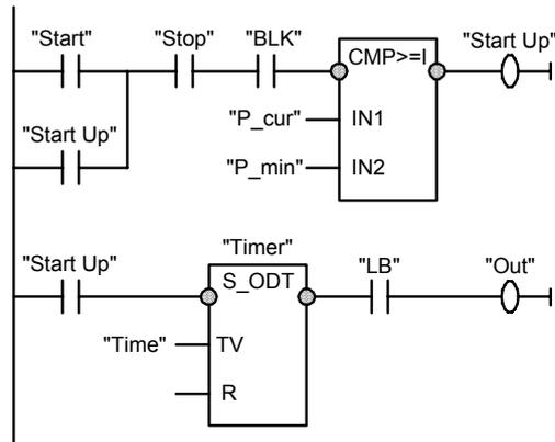
Figure 2. The ladder diagram (LD) program
