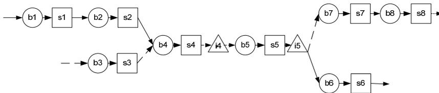
Figure 3. A family of systems with eight work stations, two products and two inspection stations after work stations 4 and 5
