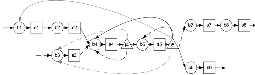
Figure 1. Multi-stage multi-product manufacturing system with eight work stations, two products and two inspection stations after work stations 4 and 5 (decision variant)
