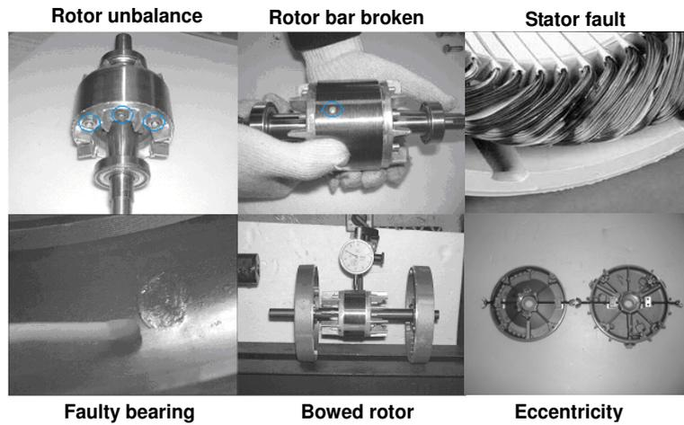
Figure 4. Faults on the induction motors
