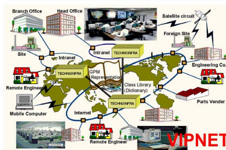
Figure 7. Distributed architecture of the Visual Production Enterprise Network (VIPNET) using Technoinfra
