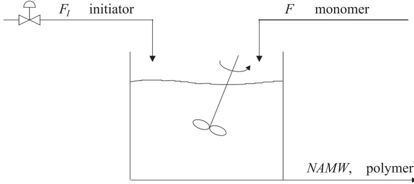
Figure 7. Polymerisation reactor
