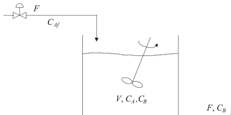
Figure 2. Van de Vusse reactor
