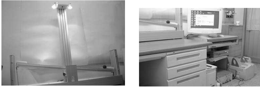
Figure 1. The AMIRA ball and beam experimental equipment
