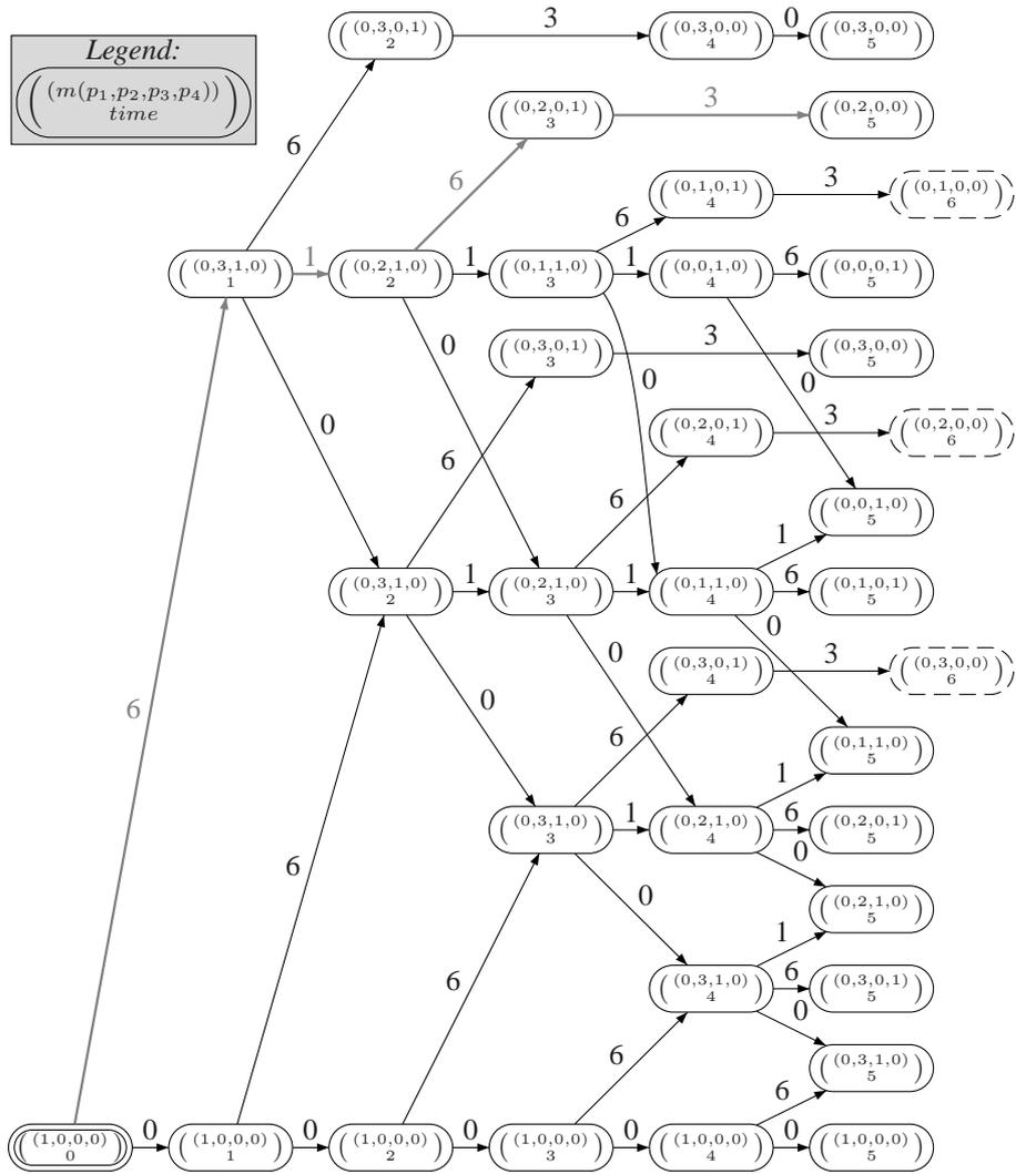
Figure 6. Modified state graph of the example system
