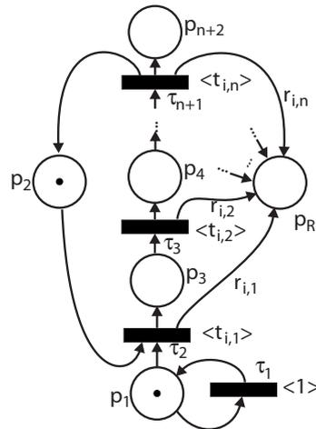
Figure 2. Non-interruptible IRIS task with reward function according to (2) without a mandantory part.
