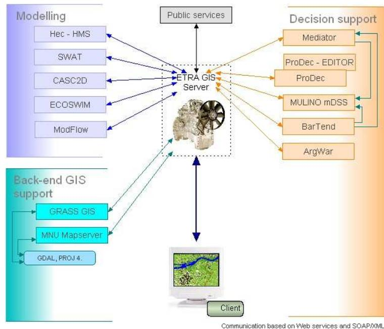
Figure 2. TDSS software architecture
