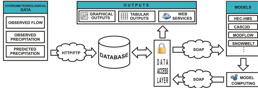
Figure 8. Data sharing in hydrological and hydrogeological modelling
