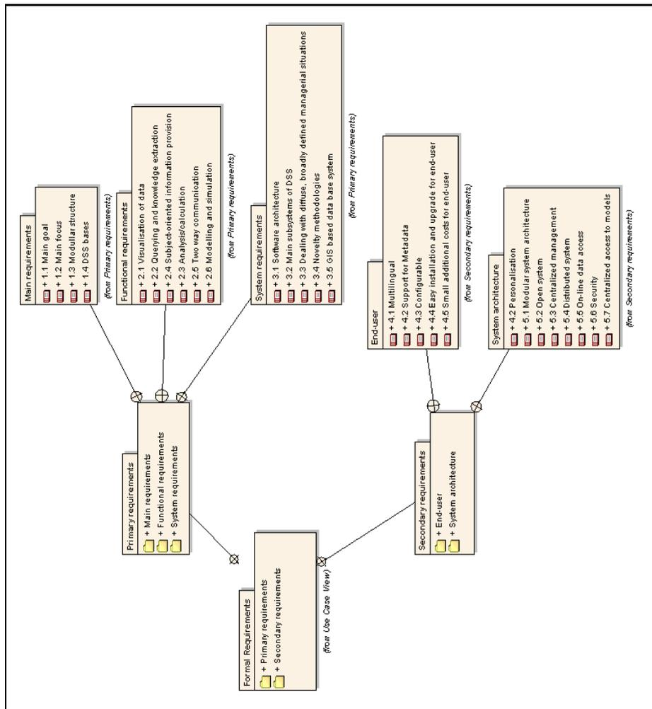
Figure 1. Classification of requirements in UML diagram
