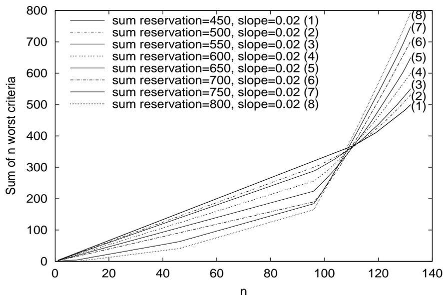
Figure 5. Varying throughput reservation for modular link capacities.
