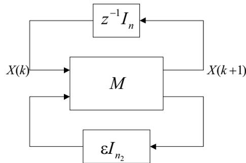
Figure 1. An LFT block diagram of system  $\Sigma_1$
