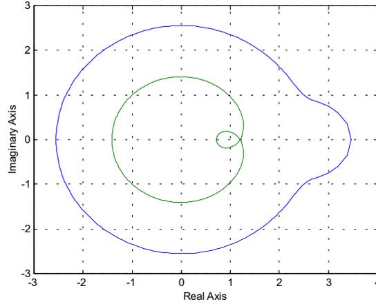
Figure 3. The eigenvalue plot of matrix  $P(e^\theta)$  for  $0 \leq \theta < 2\pi$
