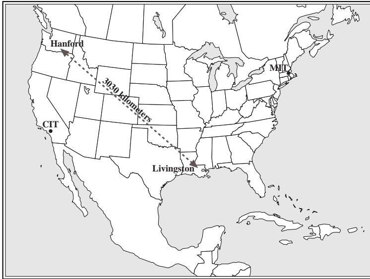
Figure 1: LIGO Sites: Two remote facilities will be located in Hanford, Washington and Livingston Parish, Louisiana. The distance between the sites is 3030 kilometers, corresponding to a maximum difference in the time of arrival of \pm 10 milliseconds for a gravitational wave.
