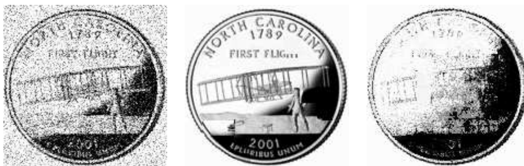
(c) Standard deviation of the additive Gaussian noise in input: 15. Reconstruction error rate — gBSB model: 0.072, hybrid model: 0.609.
